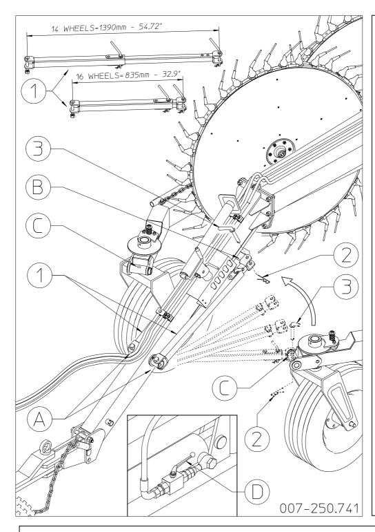
First of all, rotate the safety arms 1 from the transport position A-C to the working position A-B.
