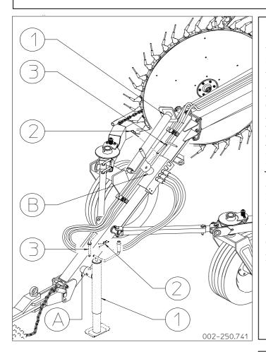
At this point remove the stand 1 from seat A (parking position) and bring it to seat B (transport and working position). To do this you must remove clip 2 and pin 3, move the stand 1 to position B and fasten it with pin 3 and clip 2.
